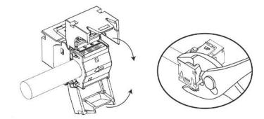
f) Insert the grounding clip, make sure the drain wire is in good contact with grounding clip, fasten cable tie to secure cable fixing and complete the installation.
