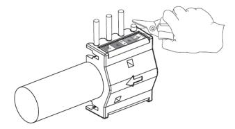
d) Follow the direction instruction on termination cap and place the termination cap onto jack properly.
