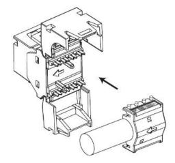
e) Secure the hinged flaps by using a plier until the flaps completely closed.
